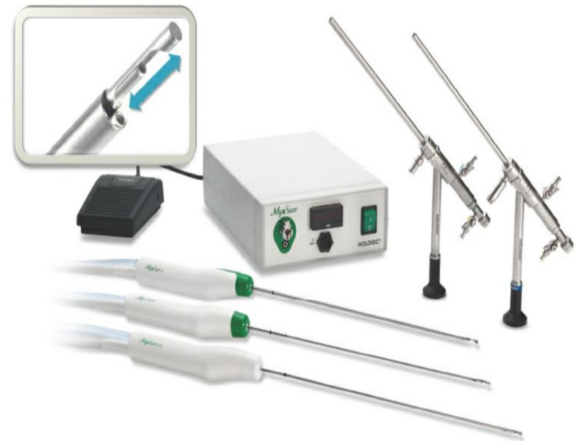
FIGURE 26-53 Electromechanical morcellator. These systems have their own proprietary hysteroscope system with an offset eyepiece (right) to allow for one of the rigid hollow probes (bottom) to be inserted. The probe is connected to a motor drive (center) that is activated by depressing a footpedal (upper left) that activates both an oscillating blade and suction. The blade transects the tissue, and the suction transports it to a collecting sac in the fluid management system.
